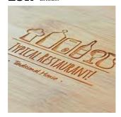
Use of a high-precision laser beam, allowing for low-relief engraving. This laser can be fibre optic, suitable for metals, or CO2, suitable for wood and cork, or UV, suitable for glass.
